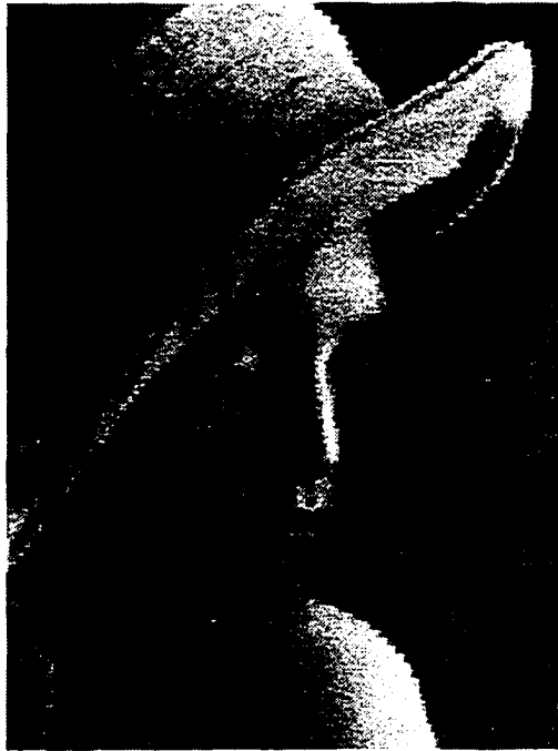
Figure 7.3: 'Staircase effect' due to vestigial edge encoding of the edge vectors (lenna - 0.254 bpp)
